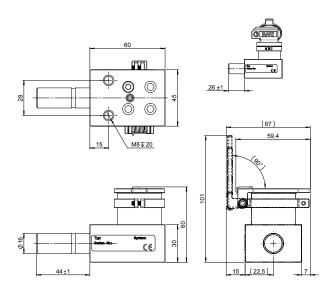
All dimensions in mm General tolerances to DIN 2768-m
