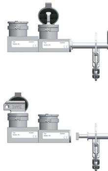
the guard locking device is closed, the personnel key is trapped
